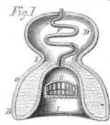
vertical section. The boiler proper, B B, is bellshaped, spherical in its horizontal section, Fig. 2, O being the outer, and I the inner shell. D is the steam dome in which the flues (only one of which is shown, at F), should expose a large heating surface. The grate, I, is placed considerably above the bottom of the boiler, a space being left entirely around be
