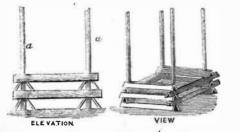
planting posts at short intervals between the corners many more boards can be stacked in the same space. This method. gives a much freer circulation of air than the ordinary method. and consequently the drying proceeds with greater rapidity.
