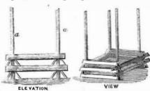
planting posts at short intervals between the corners many more boards can be stacked in the same space. This method. gives a much free circulation of air than the ordinary method. and consequently the drying proceeds with greater rapidity.
