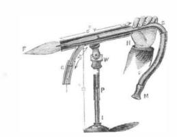
Fig. 2 is a blowpipe for light work which a contributor to the paper alluded to above, says he has used, satisfactorily, for six years. F is the flame, G is a gas tube, M the mouth piece, H the hand of the operator to draw the slide, S S, out a little for a large flame, and to compress it for a small one, T is the outside tube, into which tube, S S, slides; I is the iron wire stand; W is a gas swivel, and P the gas pipe to swivel on the stand adjustible on I.
