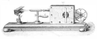
1, consists of a wood stand, A, a fan with sheet-iron frame and wood sides, B, a small driving wheel, C, and a blowpipe, D, with foot and blast tube running through its center connected by a flexible tube to the fan. E is the tube which conveys the gas to the flame, the gas escaping from an annular opening around the nozzle of the blast tube. F is a sheet-iron support for charcoal on which the article to be brazed is placed.
