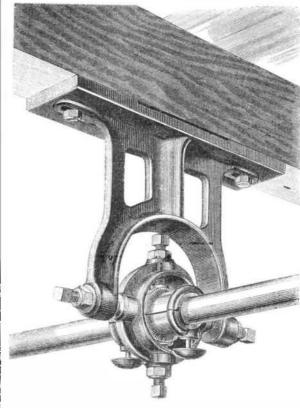
This arrangement enables the box to be made in halves and held together without the use of special bolts for this purpose, the upper and lower bolts in this hanger performing a double office.
