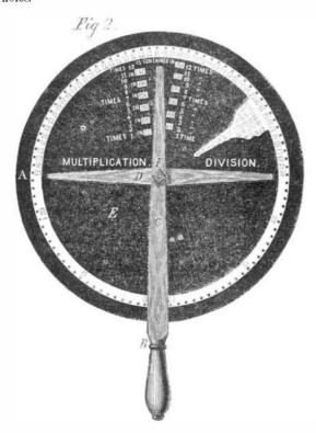
On the addition and subtraction side, the fixed disk, E, has marked on its outer edge numbers from 1 to 100 inclusive, placed at equal distances from each other, only the first ten of these being shown in our engraving, drawn in full, the rest being indicated in fives on account of limited space.
