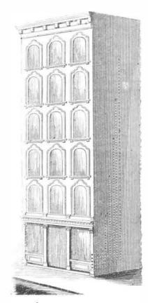
which a hose can be attached, the upper ends opening in upon the several floors above. If there is no dead wall in the front or rear, the pipes can be constructed within the partition walls (see drawing), the dotted lines showing the posi tion of pipes within the partition wall. The openings in the street need not be exposed, but may be placed in the sidewalk, inclosed, numbered, etc.
