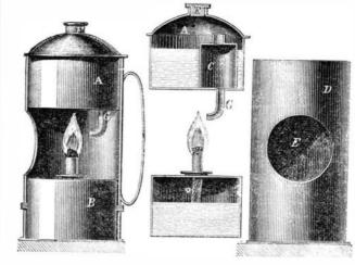
marked A has a small chamber in the inside, with a small | lution, by a pencil, into each nostril; moving his head mean in the bottom of the case, the part A is filled up to the line is forced down the small pipe,G, against the flame of the lamp with such force that it sends a strong fierce flame through the hole to the outside of the lamp. The outside hole of the blowpipe is to be made very small—so small that the point of a fine needle will only just enter.
