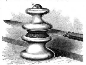
The two parts are held together by a vertical screw, B. In use the left hand grasps the top, and the bottom is pressed down upon a table. The edge of the knife to be sharpened is then drawn by the right hand through between the emery disks, the convexity of these disks, enabling a strong pressure to be brought to bear upon it, and, as a consequence, a rapid action upon the blade is secured.
