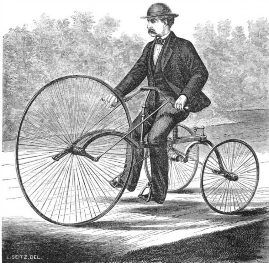
SAMUELS' PATENT HAND CRANK VELOCIPEDE.
