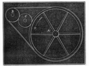
for obviating this annoyance, which we see in Engineering applied to a portable centrifugal pump. The driver, A, revolves in the direction of the arrow, carrying a belt to the driven, B, and between the two is interposed a friction wheel, C, bearing equally on the faces of both pulleys. The face of this intermediate is hollowed so that it bears on the outer edges of the pulleys. Its effect is to relieve the great strain on the shaft of B.
