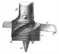
threads are cut in its surface. In a triangular slot in the head, C, is secured, by a set screw, the knife, G, which has a horizontal edge, and carries at its end the enlargement, c, which is ground to a vertical edge.
