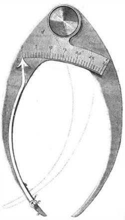
The object of the invention is the construction of an instrument that will measure objects with greater precision than can be done with the common calipers. For this purpose the index, a b, girating at c, at the end of the leg, c d, of the calipers, has its arms, a c c b, in the proportion of one to ten. The are, b c, which forms a part of the leg, c d, is divided arbitrarily into any number of equal parts, numbered as in the drawing.
