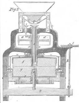
seldom happen) must be dressed by being turned round on the spindle under a stationary paint stick, which will indicate the high points and bring the face perfectly true with the spindle.
