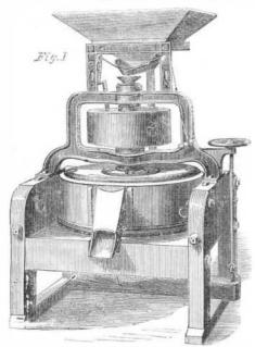
a pivot and the other end is supported by the rod, p, passing through a projection in the upper frame, and having a screw and hand wheel, I, at the top. By this means the bed-stone is raised or lowered to regulate the fineness of the grinding.
