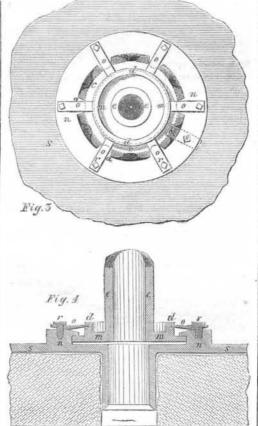
beyond the ring, d d, some distance, and the edge is accurately turned to fit the inside of the ring, n, which is cast in one piece with the cup, S. Around the edge of the plate are notches, c, which are of proper size to perhinges, which permit the upper part, with the iron frame | mit the projections, a, on the inside the river, n, to pass
