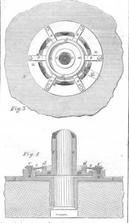
beyond the ring, d d, some distance, and the edge is accurately turned to fit the inside of the ring, n, which is cast in one piece with the cup, S. Around the edge of the plate are notches, c, which are of proper size to per-
