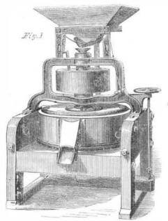
a pivot and the other end is supported by the rod, p, passing through a projection in the upper frame, and having a screw and hand wheel, l, at the top. By this means the bed-stone is raised or lowered to regulate the fineness of the grinding.
