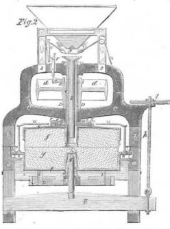
seldom happen) must be dressed by being turned round on the spindle under a stationary paint stick, which will indicate the high points and bring the face perfectly true with the spindle.
