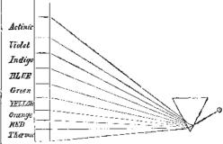
rays is admitted through a small hole in the shutter of a darkened room and allowed to pass through a triangular prism of glass, the ray is bent from its straight path and produces an image upon the wall, of varied and most exquisitely delicate colors. Sir Isaac Newton, who first made this experiment, 'pronounced these colors to be seven in number, the ray which is the least bent being
