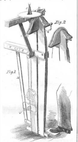
of the saw exactly over the angle in the anvil. For setting straight saws the ends of the teeth are placed against the brass guides, d d, which open at a greater or less angle, and thus permit the tooth to project a greater or less distance past the angle in the anvil.
