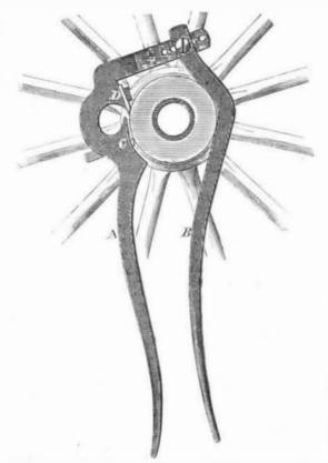
a series of holes. C is a marking or scribing cutter, and D, a chisel; both adjustable by means of set screws and slots. In operation the wheel is swung and revolved while the work, man holds the tool on the hub.
