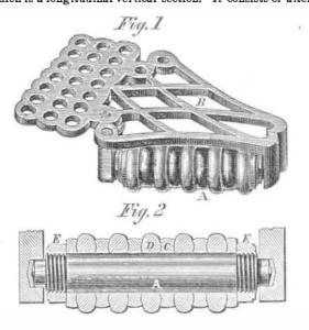
nate disks of iron, C, and rubber, D, the latter cushioned or compressed by nuts, E, at either end. As the rubber stands above the iron washer rims, it receives the pressure of the wheel and renders the action noiseless. The roller may be placed on either side of the frame, B, to suit either the right or left side of the carriage. Besides its use as a fender, it makes an elegant and handy step to the carriage.
