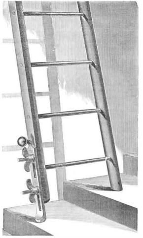
applied to both feet of the ladder, which would seem to be preferable, as it would obviate the necessity of turning the ladder to suit its changed position to the surface of the ground.
