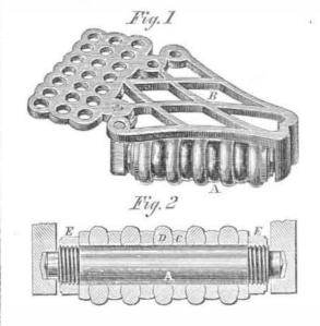
nate disks of iron, C, and rubber, D, the latter cushioned or compressed by nuts, E, at either end. As the rubber stands above the iron washer rims, it receives the pressure of the wheel and renders the action noiseless. The roller may be placed on eitherside of the frame, B, to suit either the right or left side of the carriage. Besides its use as a fender, it makes an elegant and handy step to the carriage.
