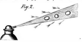
gular is the fast that the jet of steam might be inclined at any angle between the horizontal and perpendicular, and still hold the ball, egg shell, or other spherical figure, firmly in its vapory grasp, as shown in Fig. 2, C being a ball and socket X. X. to incline the jet. Syracuse, N.Y.
