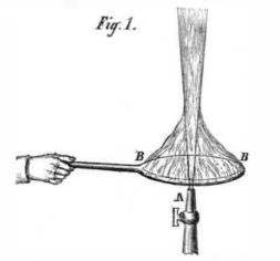
the rapidity of the blast of air moving to the steam jet." A, in the sketch, (Fig. 1,) is a steam jet, B B, the lighted torch, held around the escaping steam-the flames all rushing into the steam. Egg shells, empty flasks, India-rubber, or light copper and brass balls are suspended in the most singular manner inside an escaping jet of high pressure steam. Sin-
