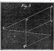
By another application of the rule of the parallelogramwe find the power, A P, parallel to the load, or the effective power to push the load along, to be 1,080 pounds, or equivalent to A Q, and a vertical power, A p, or pressure on the neck of the animal. In the same way
