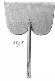
extension of the process seen in Fig. 4. Figs. 3 and 5 obviate the difficulties heretofore experienced, as they do away with the necessity of plating up the ears of the hoe before rolling. Thus prepared, the hoes come out uniform, as seen in Fig. 6, when the hoe is ready to go to the press to be trimmed and prepared for the temperer, as seen in Fig. 7. By these processes every hoe is perfect and alike.
