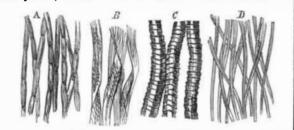
Fiber of flax, A; of cotton, B; of wool, C; of silk. D! placed so that their relative size and markings may be readily contrasted. The fiber or cells of cotton are manifestly much thinner and less resisting than those of the other substances.
