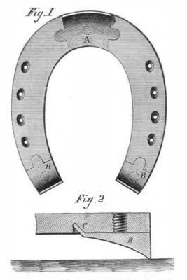
which fits a correspondingly threaded hole in the shoe, shown in Fig. 2. The toe calk is provided with two projecting pointed arms and the heel calks with one each, which after the calks are screwed in place, are bent down and seated in depressions in the under side of the shoe. See C, Fig. 2. These arms prevent the calks from casually unscrewing or turning, and tend to assist in their support, and the calks may be easily detached and replaced by others.
