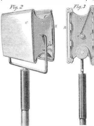
Fig. 1 shows the method of using the device; Fig 2, gives a perspective view, and Fig. 3 is a transverse section. The rectangular form of the implement allows it to work into the corners of the panes. By the use of this implement there is no necessity of climbing steps or chairs, and as there is no spilling and spattering of water it may be employed for inside as well as outside cleaning. The box can be reversed instantly to wash or wipe. Its advantages are apparent at a glance.
