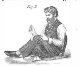
which the leg rest is adjusted. The weight of the leg is sustained by a spiral spring encircling the upright of the leg rest. The bar to which the supporting device is attached may be contracted or extended by means of a slot in the bar and a screw attached to the chair seat.
