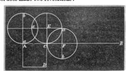
If the line, A B, is equal to the circumference of the wheel in revolving from A to B, the wheel will make one revolution, but if A B be bent into a square then the wheel will make two revolutions in passing round it.
