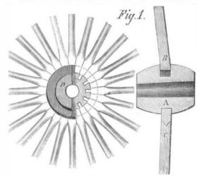
tal spokes. At the bottom of this groove the mortises for the true spokes are cut, which are seated in the usual manner, they, with the auxiliary spokes, making a solid continuation of the wheel hub, the whole being thus securely locked and fastened.
