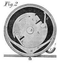
the cylinder, and passes under the wing valves through the passages, F, in the piston, which extend across its length. The steam thus admitted acts on the valves and is cut off at G, which cut-off may be increased to any desired extent by filling a portion of the steam chamber in the head between G and the induction pipe.
