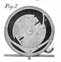
the cylinder, and passes under the wing valves through the passages, F, in the piston, which extend across its length. The steam thus admitted acts on the valves and is cut off at G, which cut-off may be increased to any desired extent by filling a portion of the steam chamber in the head between G and the induction pipe.
