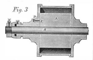
tion of the engine is shown by the arrow in Fig.2. In Fig.3 is seen a collar, M, screwed on the end of the shaft to prevent the pressure of the steam, which is admitted at that end, from forcing the piston against the opposite end of the cylinder. This collar forms a joint with the stuffing box.
