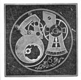
count of first being made for China, so that they could see the watch go plainer than by having a small seconds hand. They are made with the duplex escapement, and having a very large balance. The inner back of the case is generally glass, through which all the works can be seen. The brass works are ornamented with engraving, which with the bright and
