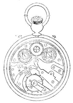
These watches were used principally for "timing" at races etc. By their use the time can be taken to a great nicety This is done by means of a small thumb piece, at the side of the case, which either starts or stops the one quarter or one fifth seconds instantaneously, without disarranging the true time of your watch, no matter how often you stop or start it.
