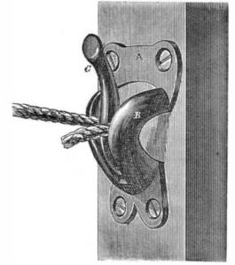
cast or malleable iron, with two bows, B, spreading from the bottom up, and having their inner surfaces beveled from the outside inward. Between these is a tongue, C, pivoted at the bottom end and shutting in between the jaws, B. This tongue is also beveled, its lower edge being the thickest.
