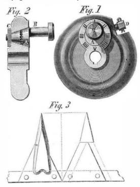
The part, A, or shank of the wrist pin, B, which enters the wheel, is tapered as shown in Fig. 2, the wrist being placed near the periphery or eccentric to the center of the shank. The projection of the shank on the back of the wheel is square, having a square washer, C, by which the wrist pin and shank can be turned toward or from the center of the wheel, making the stroke shorter or longer, marks on a dial seen in Fig. 1, showing the relative positions of crank pin and center of wheel.
