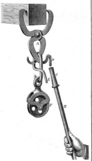
any ordinary blacksmith and cannot easily get out of repair. The patent issued to G. W. Gregory is the first one taken out for clutch or adjustable pulley support, to be operated by use of poles, and his patent covers the device of elevating the clutch by means of a pole.
