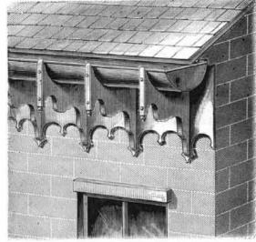
eaves, and the front by strips of metal secured to the front edges of the brackets, and provided with a hooked end to embrace the edge of the gutter. The result is a neat and secure device for supporting eaves gutters. The attention of builders and others is directed to this economical and efficient device. Territorial and manufacturing rights are for sale by the patentee.
