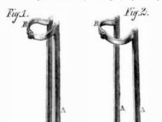
2 shows the tongs open, and Fig. 1 embracing a crucible. The elasticity of the bars when compressed by the hand will cramp the segments around a crucible with sufficient force to prevent it slipping in the tongs when canted to pour the metal.
