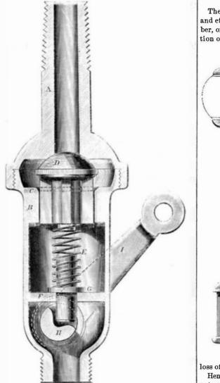
ing screwed into the cylinder, the steam presses down and closes the valve. D. until the steam in that end of the cylinder "exhausts," when the valve immediately opens and allows the water to escape, thus leaving a continual opening in the cylinder, but without the escape of any steam; should it become necessary, the valve is raised by moving the handle, I.
