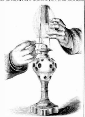
top. It has its advantages in giving excellent support to the glass while the lamp is being moved about and in the ease with which it can be lifted, as shown in the engraving. The edges of the flame, always the hottest portion, are directed against the metallic uprights, which thus defend the glass from inteuse heat, and the upper portion of the glass is adapted in its inside diameter to the outer diameter of the metal top, so that the draft of thechimney is not impaired.
