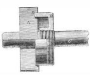
cured, as usual, by a key, all mechanics know that it is very difficult to set a cutter twice alike; and the notch, which is filed in the cutter, to prevent it from moving endways, is a great source of weakness, often causing the cutters to crack in hardening, as well as after
