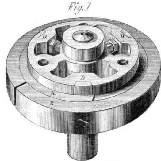
themselves to the varying pressures of the steam on the piston. A number of attempts have been made to produce a self packing or steam expanding piston, which will act always with the pressure of the steam and the velocity of the engine. The advantages of such a piston will be readily ap-
