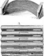
sections may be made of any length or width required, and may be held to the ceiling or walls by nails or screws. For he latter, where strength is required, thicker iron may be employed in combination with iron flooring beams, as seen at B. It can be used for clapboarding, lining, siding, or roofing, as may be required, rendering the building absolutely fire proof, and immensely stronger than any brick or wooden structure. These do not exhaust the uses of this
