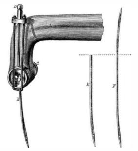
placed over it, and held by a piece of elastic cord as seen in the engraving. E and F show respectively the ordinary single needle and the improved double needle with their relative
