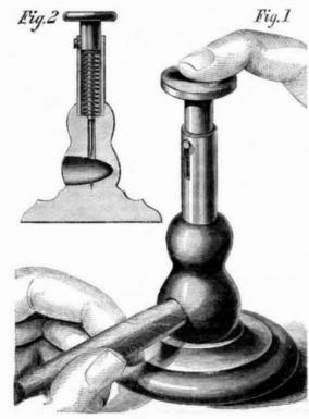
top of the stand rises a sheath in which a piston moves, car rying at its lower end a needle of proper form for puncturing the cigar, and having at its upper end a button to receive the pressure of the finger or thumb.
