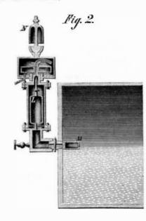
This alarm device consists of the single valve, L, whereby the orifice of pipe, M, is kept closed as long as the water stands above the dotted line, but is opened as soon as the wafalls below the line, to allow the steam to flow through pipe. M, for the purpose of blowing an alarm whistle, N. The apparatus is represented in Fig. 2 in the state of allowing the steam to flow through it, for the purpose of blowing a whis-
