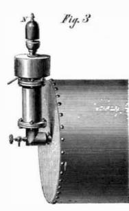
This device can be put on outside of the boiler, and its proper place will be at the point of the middle gage cock. It can be put on in place of the middle of the three gage cocks, and the middle gage cock again put on the bracket of the alarm device. The bracket can be provided with a stop-cock. This device has been in successful operation at different places in Philadelphia. Patented June 4, 1867.
