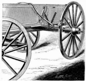
It is simply a sleeve or cylinder on each side of the team, near either the front or hind wheels, and turning on a shaft fixed to the body. To this cylinder is attached a properly shaped shoe formed so as to engage with the wheel, either on a curve corresponding with the circumference of the wheel, or on a curve which gives it a cam shape, so that when the pressure is upon the wheel the resistance of the brake or shoe shall correspond.
