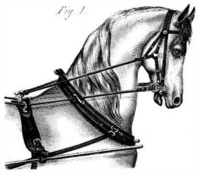
cure the occupants of a vehicle from the dangers of hard-bitted and fractious animals. The two engravings show the construction and action of an improved rein patented by Joseph C. Haines.
