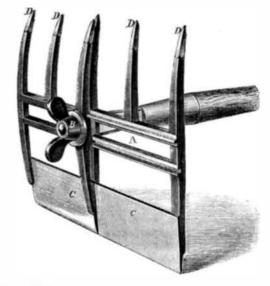
bars of which are rabbeted to receive the slides of A. Each frame has a steel blade, C, and rake teeth, D. When fully extended, the two blades form one of considerable length, and the rake is open, as shown in the engraving. If the outer frame is slipped half the distance between the teeth, it makes a narrower blade and a rake only one-half as coarse as when fully extended. The whole frame can be secured by the center or near either end. Any adjustment desired can be made instantly.
