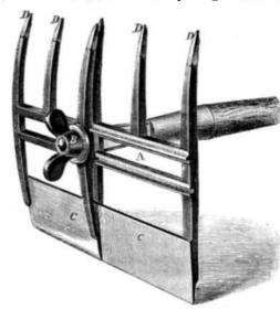
bars of which are rabbeted to receive the slides of A. Each frame has a steel blade, C, and rake teeth, D. When fully extended, the two blades form one of considerable, length, and the rake is open, as shown in the engraving. If the outer frame is slipped half the distance between the teeth, it makes a narrower blade and a rake only one-half as coarse as when fully extended. The whole frame can be secured by the center or near either end. Any adjustment desired can be made instantly.
