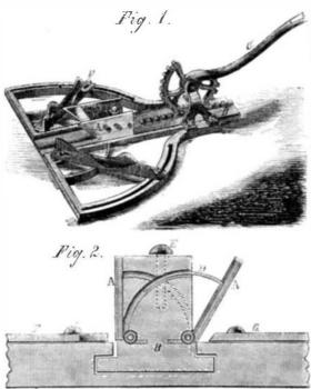
knives are adjusted in the position seen at F, A, in both figures, and by adjusting the rest the end or edge can be cut to any angle desired. For mitering flatwise the position of knives and rests is as at G, A, Fig. 2, the rest being secured at an angle of 90° with the cutter head and the knife, A, being brought and secured in the desired position.
