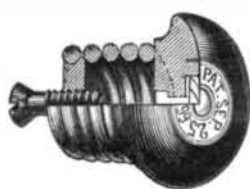
Fig. 1. shows one of the forms covered by the patent, which can be applied to old as well as new stoves. It consists of a heat-radiating coil, fastened at one end by a disk and screw to the door, the other end being riveted to a wooden handle. The same contrivance
