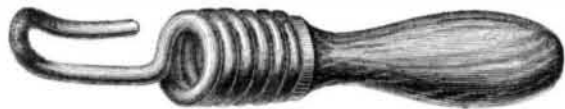
Fig. 2 shows a lifter for covers, made on the same principle, which can be easily fitted to any size or form of groove.
