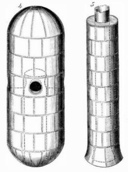
the tubes or flues, the principal advantage being in reducing the quantity of water in the boiler which is acted upon by the fire.
