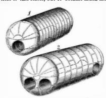
when the cylindrical boiler usurped their place. One of these is seen in No. 1 with a tube passing from the rear of the fire to the front of the boiler. No. 2 has two tubes which open at the front and at the sides near the rear end. Both these are externally fired. They are extensively used now
