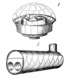
proved by increasing its heating surface by constructing a central dome-like fire place with a curved flue conducting the gases of combustion through one evolution within the boiler before passing around the outside. It is shown in No. 1. The dotted lines show the exterior form of the boiler. Its construction, although improving the boiler for a steam generator, greatly weakened its strength.
