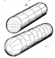
The object of increasing the strength of boilers by diminishing their diameter led to the construction of boilers of a cylindrical form. They, however, had flat ends generally of cast iron, as are hundreds still in use in this country. The flat surface has much less resisting power than a convex surface, and as cast iron will not yield much without breaking, the blowing out of the boiler head is the usual form the explosion takes in case of accidents to this class of boilers,
