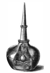
silver plated, for the sewing machine, and weighted at the bottom, as at B, to bring it to an upright position when accidentally overturned. This is further assured by the form of the can. For common purpeses the oiler can be cheaply made by constructing the lower section, from the line, C. of cast iron. thick as seen at D and B, which would further insure steadiness of position by increased weight.
