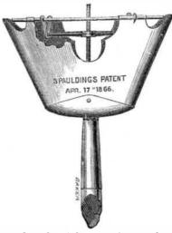
is turned to the right, screwing up the arms and contracting the sides, when the broom is clamped tightly between the sides of the shell. It seems to be a very efficient device for the object sought.
