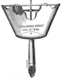
is turned to the right, screwing up the arms and contracting the sides, when the broom is clamped tightly between the sides of the shell. It seems to be a very efficient device for the object sought.
