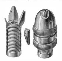
proper drill chuck, adapted to all sizes of drills and demanding only perfectly round chucks, is quite modern. Yet these chucks are considered now an absolute necessity in every well ordered shop.
